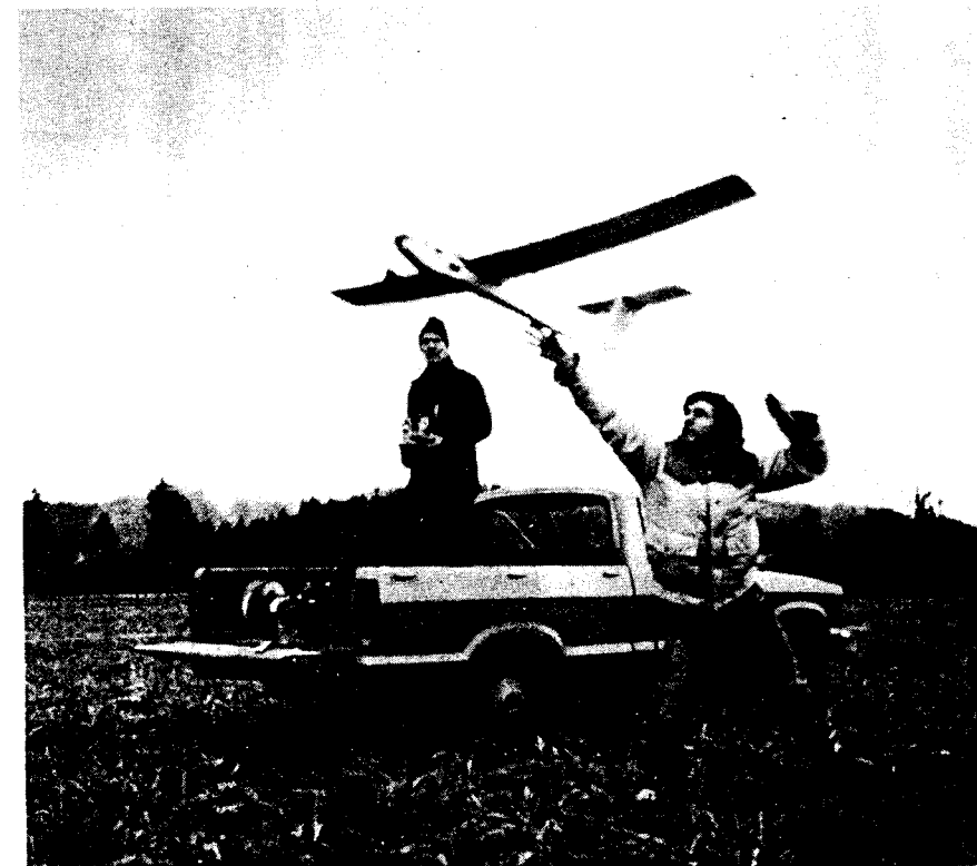
WING-STEERED SAILPLANES ARE BECOMING MORE POPULAR. THIS 2-METER DESIGN BY JIM BROCK USES PARTS OF OTHER SAILPLANES. NOTE WINCH ON TRUCK IN BACKGROUND...NEAT IDEA. JIM AT CONTROLS. HELPER LAUNCHES.
