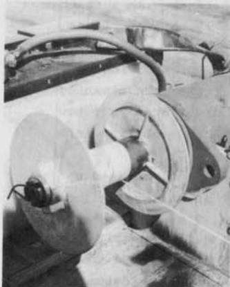
Winch drum - two large pulleys and TV mast hub; Top view shows copper strap between battery and motor case
