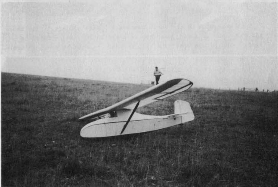
The cute little Hutter 17 awaits its tow for another flight. Original used bungee launch (no wheel) and weighed a mere 250 pounds! Many pilots said it was a delightful sailplane on the slope or in thermals. Speed was about 30 mph! Charlesworth model.
