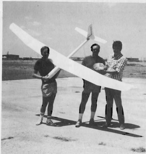
Winning Team: Joe Wurts, Greg Baker, Gary Ward. Airplane is "Wile E's Revenge" with glass wings and fuse, Eppler 374.
