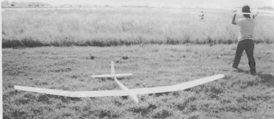
Chuck Caldwell's Merlyn, Sealy fuse, Selig 3021 airfoil- a real floater at 11 lbs., max area.
