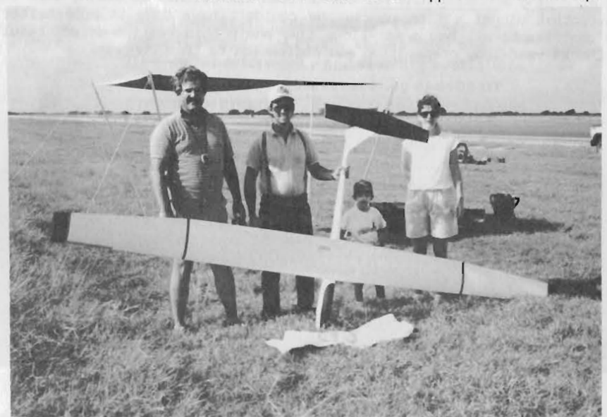
Dick Roddy Jr., Jim Ferris & Family. Formica® over foam on an Eppler 374 with flaps
