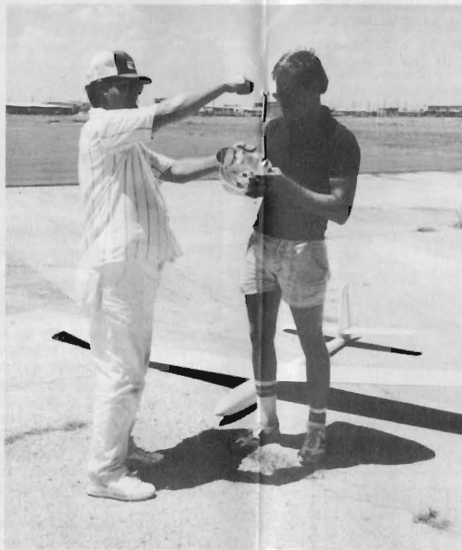
Winning Team: Joe Wurts, Greg Baker, Gary Ward. Airplane is "Wile E's Revenge" with glass wings and fuse, Eppler 374.
