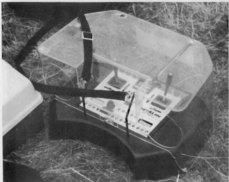
Radio with "Sender Saver" rain guard
