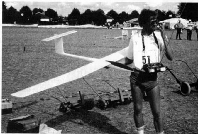
Nic Wright, Great Britain 1989 F3B World Champion. The model is the ELECTRA E1 with an RG-14 airfoil trimmed to 7%. Wing skins are all carbon fiber laminate. Photo by Terry Edmonds.
