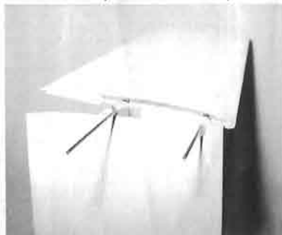
3/8" aluminum rod is glued to the rudder post.
