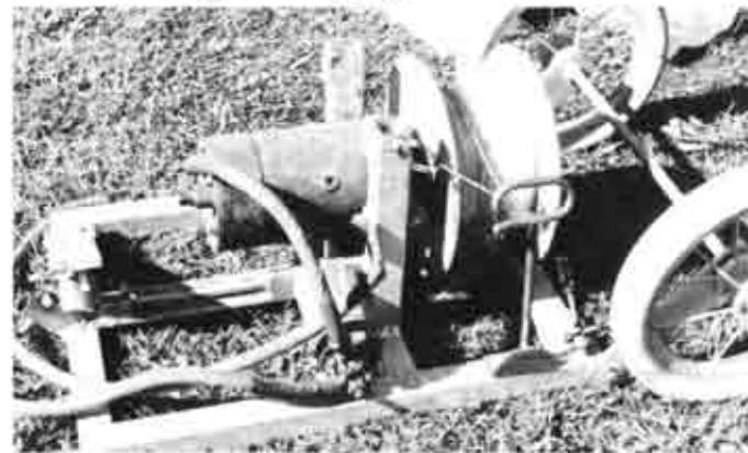
An overall of the winch that clearly shows the foot pedal, the solenoid actuating arm and the solenoid, itself. Club winch made by Bruce Abell. Photo by Bruce..
