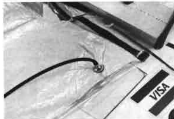
Aerospace Composite Products EZ Valve installed in bag for use.
