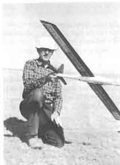
Photo 3. Frank Deis holding the Talon ready for launch. Note the forward location of the tow hook. I glued some 400 grit sandpaper to the rear of the fuselage to keep the Talon from slipping out of my grip.
