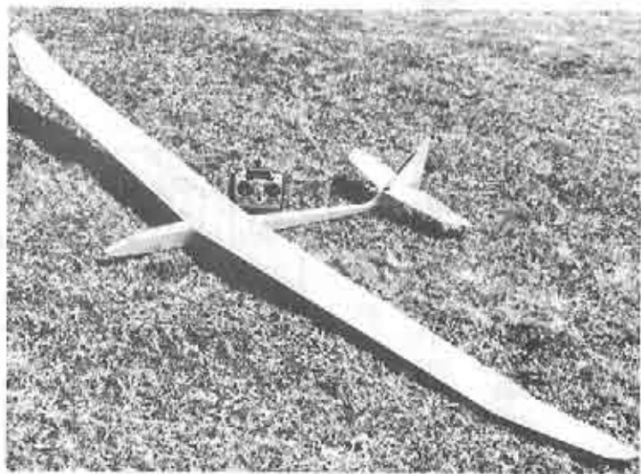
Wingspan: 121", Wing area: 975 sq. in., Weight: 60 oz., Loading: 9 oz., Airfoil: SD7032/7037
