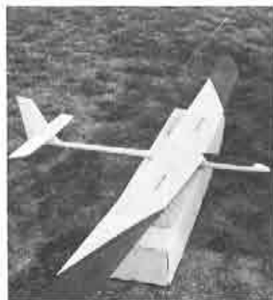
An especially fine specimen of a Falcon 880, built and flown by Peter George, from St. Louis. Peter painted on the neon tips and black stripe, and used regular Magic tape to secure the flaps and ailerons.
