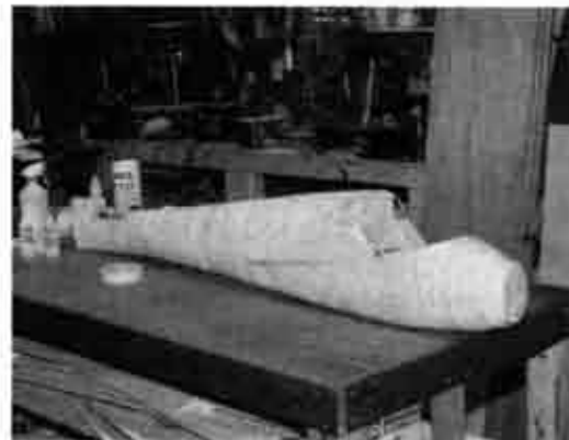
Photo 7 - Fuselage is epoxied together and held in place with tape and rubber bands.
