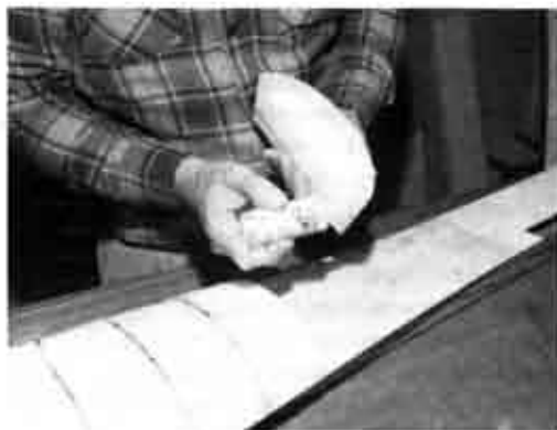
Photo 4 - Use CA on the balsa and spray adhesive on the foam to glue form on the plywood.
