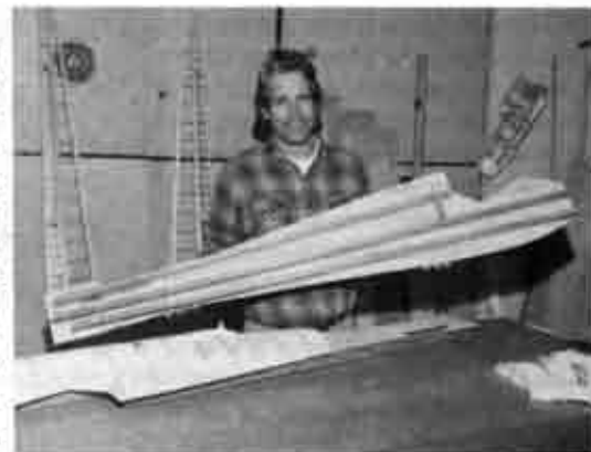
Photo 1 - Rusty Hupy holds up fuse profile showing 1" x 2" stiffeners spot glued on back.
