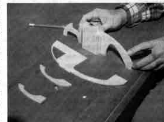
Photo 2 - Formers, including former with wing rod tube installed.
