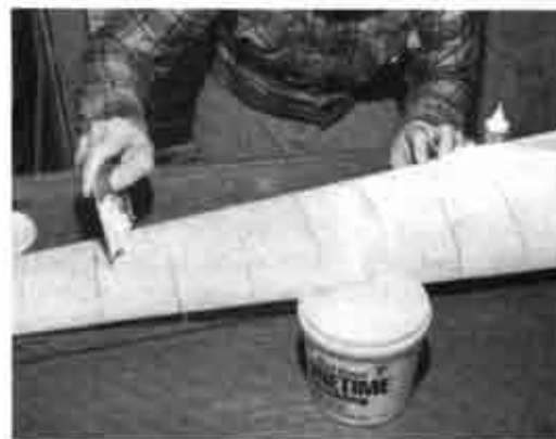
Photo 5 - Light weight spackle works great to smooth out foam and fill in wing fairing.
