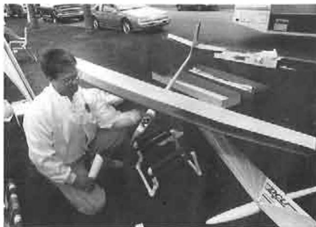
Mark Hamblton of DCU shows his new 2M & Unlimited entries in the thermal duration arena. Both ships are prototypes and will be kitted, soon. Both use foam/balsa 7037 wings with Mark's great glass fuses.
