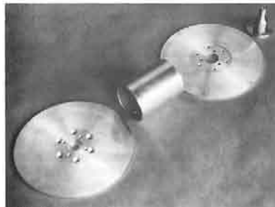
#3 almost ready to go. Brake arms are machined from solid aluminum stock and line guide is aluminum tent stake.
