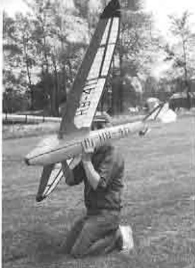
Spalinger S-18-II modeled in 1:4.5 scale from 3-views in "The World's Vintage Sailplanes" by Martin Simons. This particular model was modified from the original by Willi Schwarzenbach (Switzerland) by lowering the wing pylon and modifying the cockpit canopy (less drag). Scale model designed and built by Gerry Knight and held in this photograph by Cliff Whybra of Niagara Falls, Ontario.
