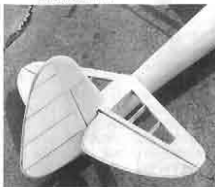
Rudder and tailplane assembly in one piece. Keyed and one bolt to rear of fuselage. Note that all ribs are stained to simulate spruce originals. Covering is "Solartex" antique with a coat of clear or "Glasscoat".
