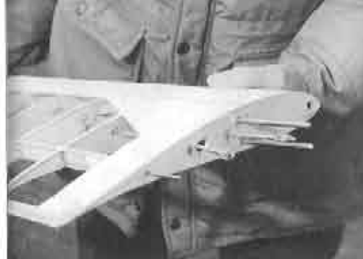
Wing root - section, Wortmann FX-1261. Note the two wing rods vertically mounted at the main spar. Since this picture was taken, the aileron servos were installed - one in each wing. The spoiler servo is in the fuselage. Wings are retained to fuselage pylon by big elastic bands. All my big birds have the dual vertical wing rod system which is very strong (and successful).
