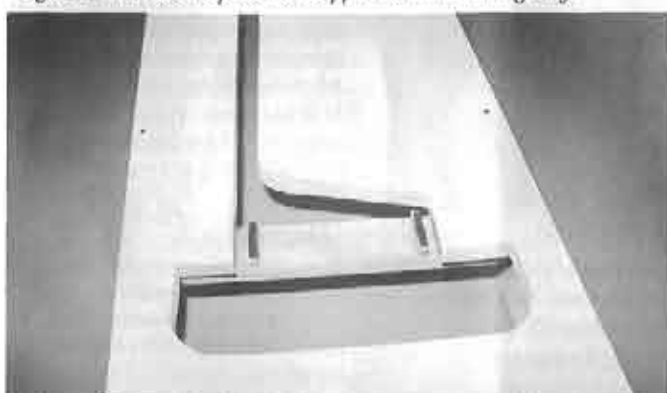
Figure 6 The rudder is provided support with modeling clay.
