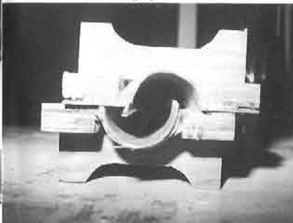
#5 - When joining the two halves together, start with the mold halves off center and the tails sticking free and clear.
