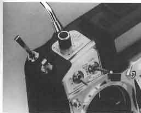
The upper left corner of the X-388S Tx is the location for key function switches. The 3-position switch directly above the left stick is for the Launch and Reflex Pre-sets. The switch near the front on the top changes the "mix SP" function from camber to landing mode.
