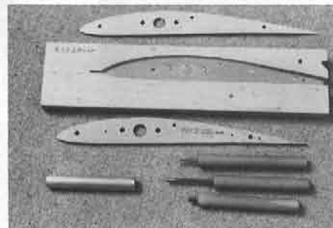
Rib drilling jig & hole cutting tubes A/ Balsa blank drops into jig B/ Ply rib locates over balsa rib C/ Balsa rib drilled through ply rib template using sharpened tubes
