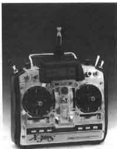
Front of the new X-388S Transmitter from JR. Switches for mixes and pre-sets are optimized for sailplane use.
