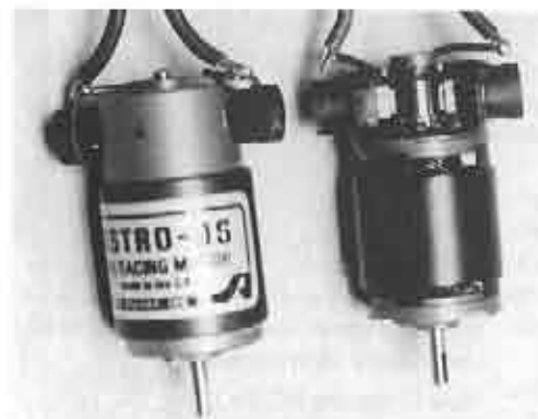
(R) Modified motor from Kirk Massey, (L) stock motor
