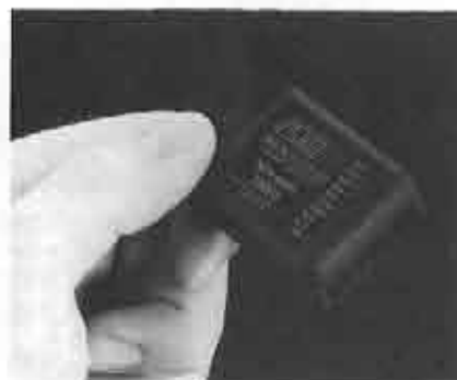
The 649S receiver. This uses the new 5-PCM and is extremely compact for a 9-channel receiver. At only 1 ounce in weight it is the smallest and lightest 9-channel receiver made.
