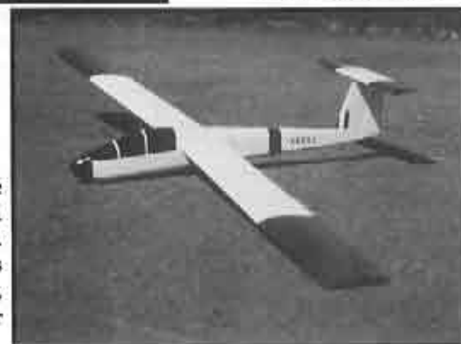
Gene's finished T-53 is waiting to fly. It uses a Quabek 3.0/10 airfoil.
