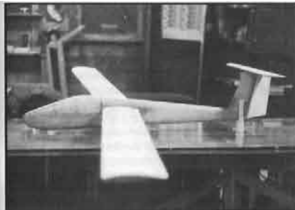
T-53 sits on workbench ready for paint. Model employs blue foam core wings with obechi skins. Fuselage is glass which was made over a foam plug.
