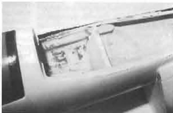
Photo 2 - Inside of fuselage. Shows former, pushrods and paint, which have to be removed.
