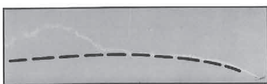
Figure 4 - Smoke path for a small bubble thermal approximately 20 seconds after flying through it. (Dashed line shows original flight path.)
