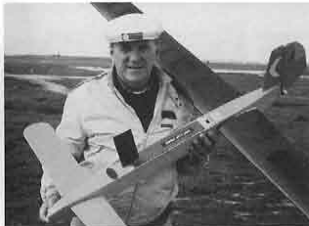
Mark I uses Windfree wings, too-small canard and short-coupled rudder. I even tried a front rudder to get better turning.
