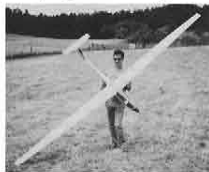
1/4 ASK 21 built by Jack Kagi from a Rodel Modelle kit. Flies beautifully! (4.2m. 5 1/2k.)
