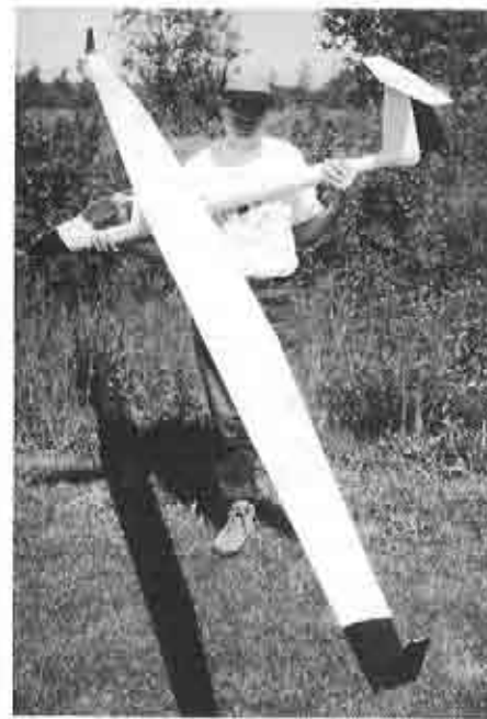
Ron Wahl holds a 1/5 SB9. 9 lbs., 4.4m., built from a Kraus kit. Note the winglets!
