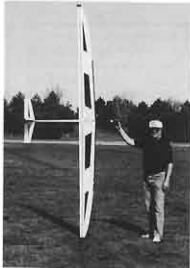
Note the bagged-in color scheme on top of Genie #3. The bottom is black with the same markings in white and red. I don't know if anyone else has tried the paint trim techniques used here, but it is not difficult and results in a ridgeless transition between colors and no pin holes.
