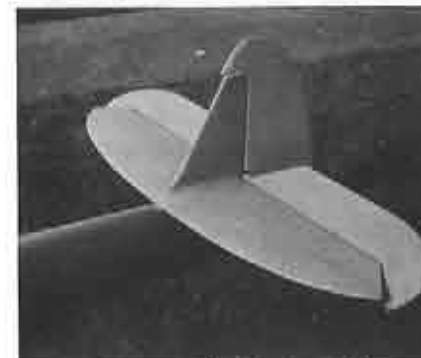
Monokote covered and primed (laquer grey auto primer). Ready for final painting and detailing.
