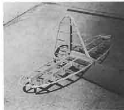
Built up tail feathers ready for covering.
