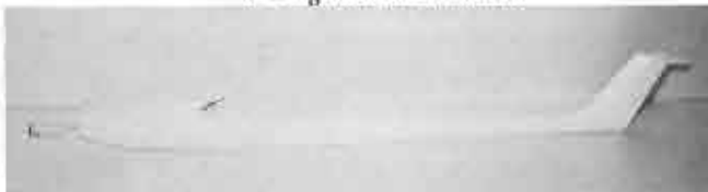
8. Finished plug with wire loop added, so that it can be hung while being painted.
