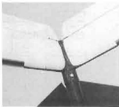
Top view of Magic "V" tail before glass tube was added.
