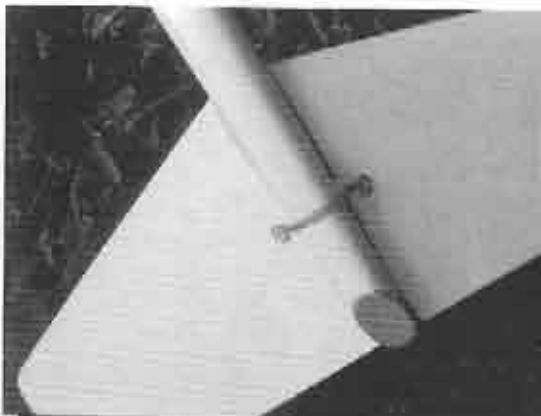
V-tail pivot wires glued in w/wood blocks inside fuselage.
