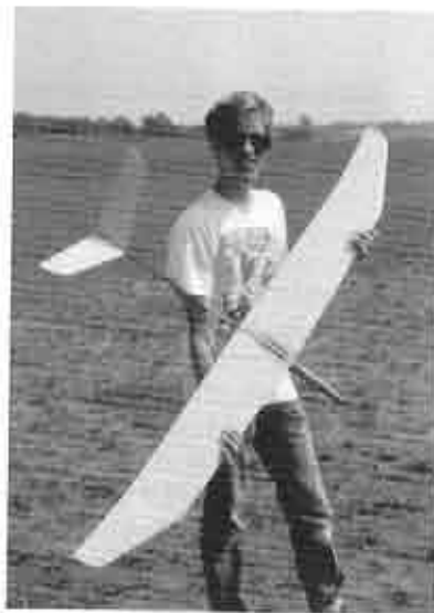
Cody Robertson and his O/D called the AeroBat. Fiberglass pod and aluminum arrow shaft boom. Cody developed his own airfoil for the model and the sheeting is basswood. Note the swallow tips.
