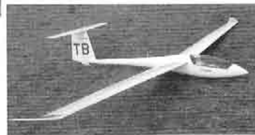
Terry Luckenbach's Unlimited ASW-20 flown by him to 10th place. Note the "tailhook" skeg at the base of the fin.
