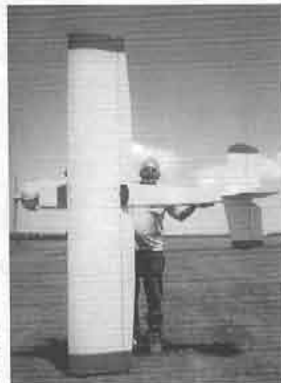
Photo 4 - Enlarged Robin 99 with a Quadra 100. Weighs 25 lbs.
