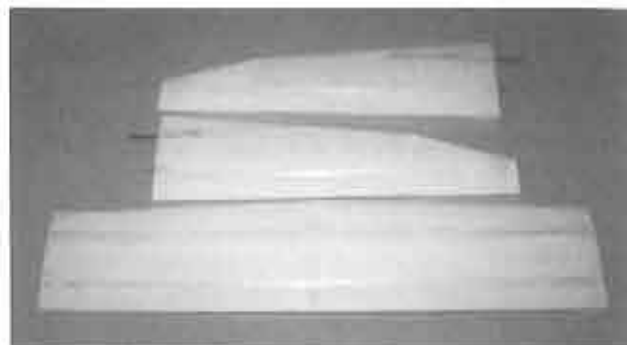
#4 Completed foam cores
