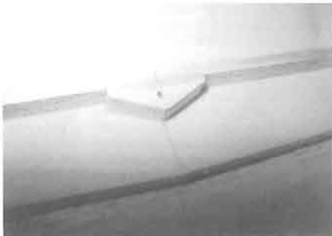
#3 Hard point glued onto spar
