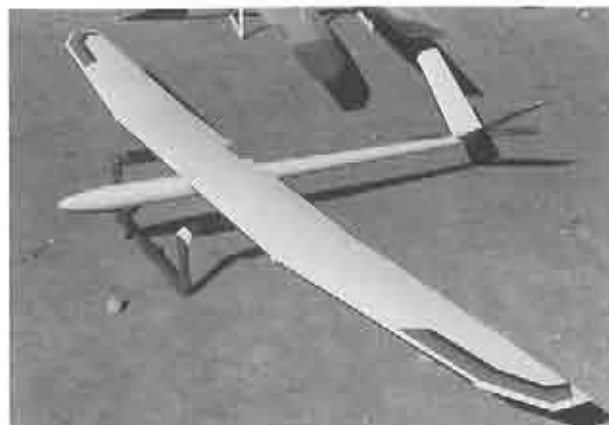
Fredo, F3B design, RG 15, 114" span, 85 oz., 12.2 oz/ sq. ft., 1000 sq. in. area. There were three at the Southwest Winter Contest. Molded ship by Fred McClung of Albuquerque, New Mexico.
