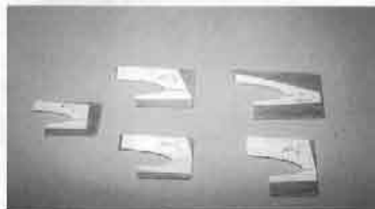
#6 Templates used to shape leading edge.
