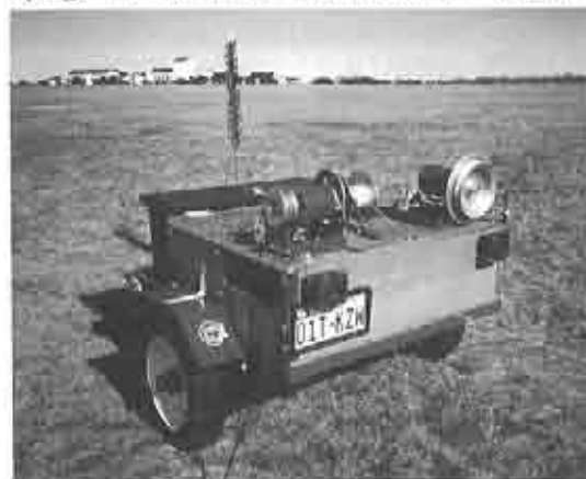
Business end of trailer mounted Rahm winch and retriever. Editor ran this system at '93 TNT contest. It is a reliable, consistent, work house.
