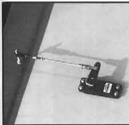
Aileron servo in the wing.
