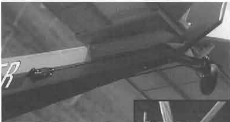
View from below. Rudder and elevator servos are in the tail.
