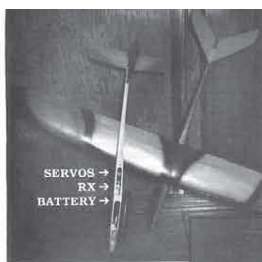
(L) Blu Dartar fuselage. Note radio location. (R) Weston Aerodesign Co. fuselage. Both planes are set up to use my Epsilon wings.
