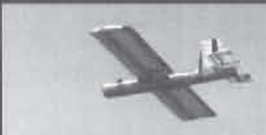
A slightly modified "Carnagesaurus". Notice the fins have been moved into the fuselage. Also, notice the use of a slaperon setup. Camber changing can be very useful in combat flying, allowing you to stretch a given plane's envelope considerably.
