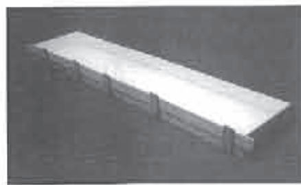
Wing is installed in parting tray. Note trailing dam is held in place with clamps.
