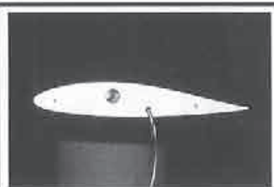
Ripo 1/3 DG 600 Root Section The trailing edge actually curves up! The model has flaps, ailerons, and spoilers.
