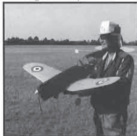
Eut Tileston with his Stahl scale Caudron Fighter for Spirit of SAM event. It was flown by Kirby Hinson, and performed very well. Graupner Speed 400 with Simprop gearbox 5.9:1.
