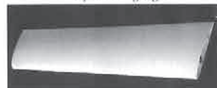
Completed wing removed from mold.
