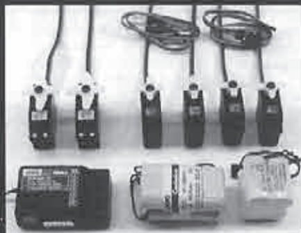
Control system parts prior to installation: JR NES-3021 mini servos for elevator and rudder and JR NES-341 servos for flaps and ailerons, RCD 3600 receiver and Sanyo 600 or 250 mAh battery packs, depending on final balance.
