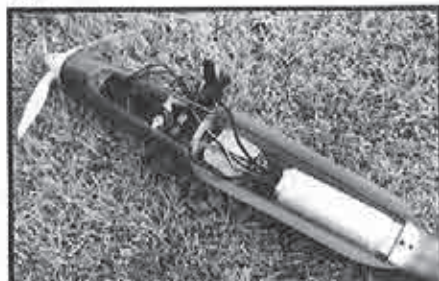
Up front is the Graupner Speed 400 6V motor with JETI JES-10 speed controller attached to the back plate, followed by two HS-60 servos. Behind the bulkhead is a lightened JR credit card receiver and a 7 cell 500AR motor pack. Yes, it all fits!!
