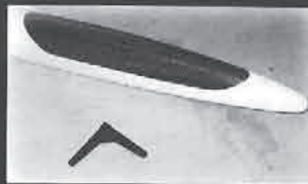
Condor fuselage with custom designed bellcrank - plastic injection molded.
