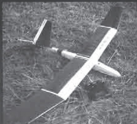
Midwest Essence: two piece wing, simple joiner, ample spoilers, and tough spar!
