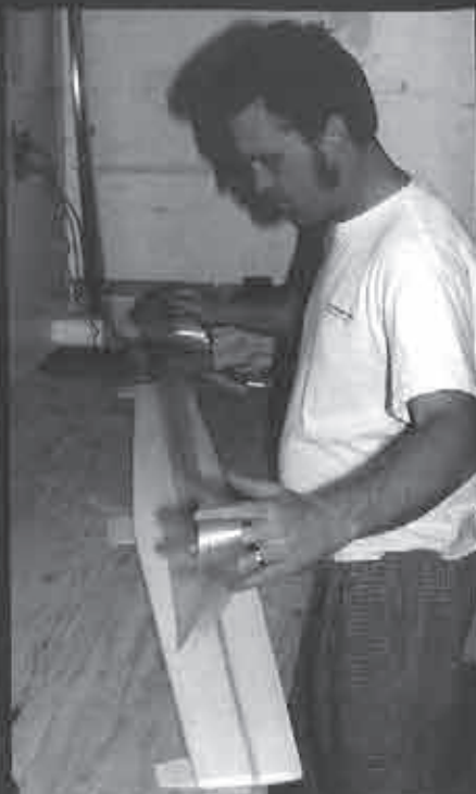
Here, I'm laying a long strip of tape on the top surface of a wing. By holding the ends and letting the middle drop down onto the panel in a gentle arc, it's easy to maintain control of the tape while laying it on smoothly.
