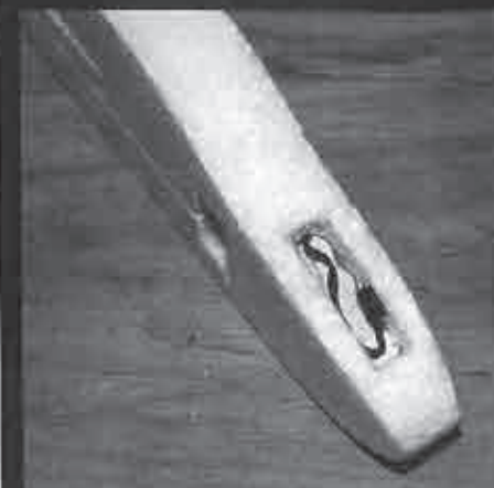
The battery compartment in one of my foamies. Notice that I've cut the cavity so the battery fits well below the surface of the fuselage. A foam plug will fill the hole and be cut away as required to install a switch and to access the charging jack.
