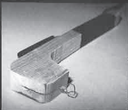
Hand held, hot wire conduit cutter.
