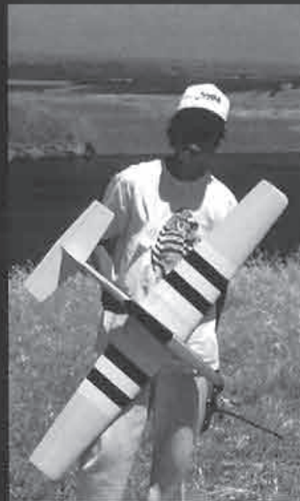
Mickey Crowley and his scratch built Mustang. 48" span, 16 ounce model was a hot performer in Mickey's capable hands. Wings are un-sheeted blue foam with low temp covering.
