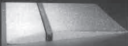
Spar glued to back half of foam core.
