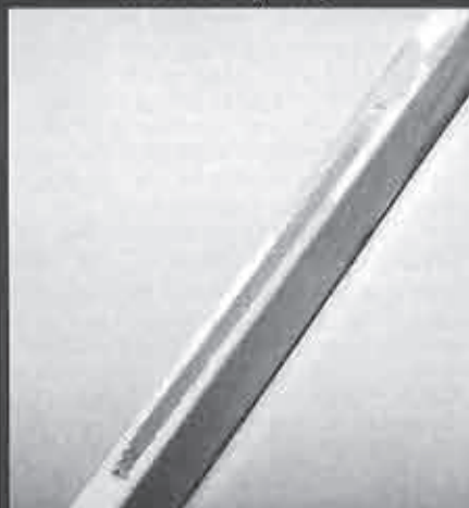
4 inch by 1/8 inch hole cut from top to bottom of spar. This is the polyhedral break, which we'll talk about later on.
