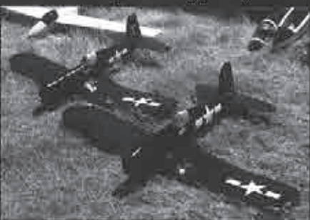
Aerofoam 49" span EPP Corsairs on the ramp at Los Banos '97. These planes were very impressive and ingeniously designed, with combat and rough sport use in mind. The foreground plane is missing its EPP spinner cone, which attaches with velcro. Shelby Sanders photo.
