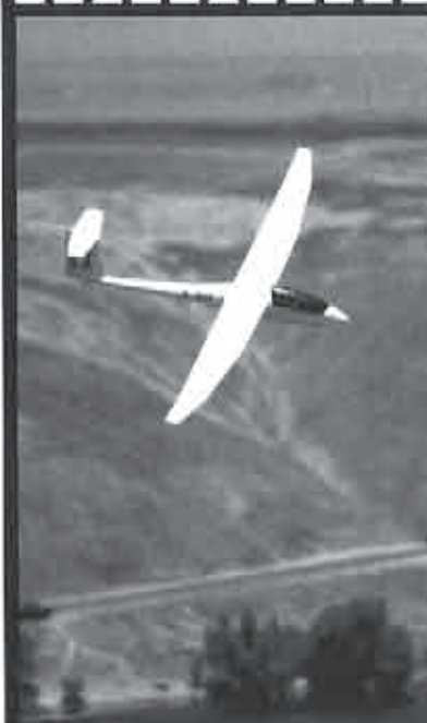
Gary Brokaw's 1/4.4 scale Discus. Graupner fuse, and 5% overscale wings.
