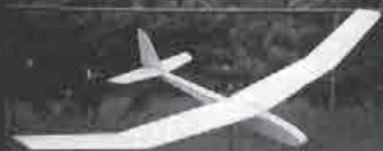
Torque & Recoil Club's 'Bob'. Middle school styrene foam and ply construction are used to create a very light and strong performance HLG at a very reasonable price.
