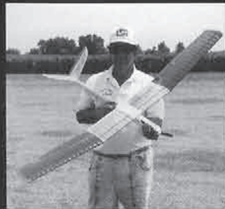
Dave Grife from Michigan with his DH Mosquito from Brian Taylor plans. Two Astro 25 cobalts with AFI's new super gear box. 35 - 2000mah cells and ALIW of 14 lbs. Model is over 4 years old and still flying strong. Not a hangar queen!
