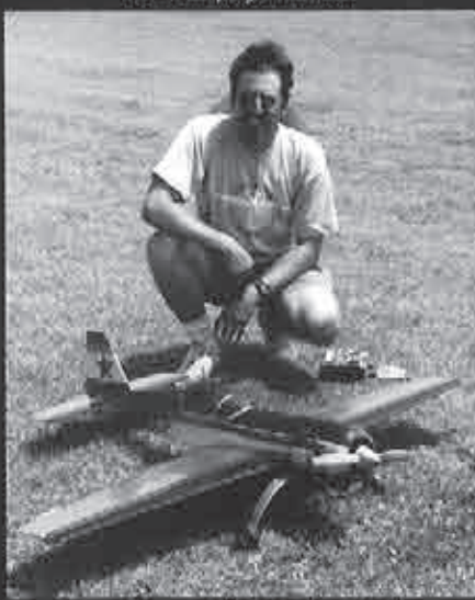
Peter George of St. Louis with his Graupner Sukhoi Su-26M. Model uses Graupner Ultra 1600 with a 2:1 belt reduction, Astro 210 speed controller, and 16-1700 mah cells. Model has plenty of go and can do full aerobatic routine with ease.
