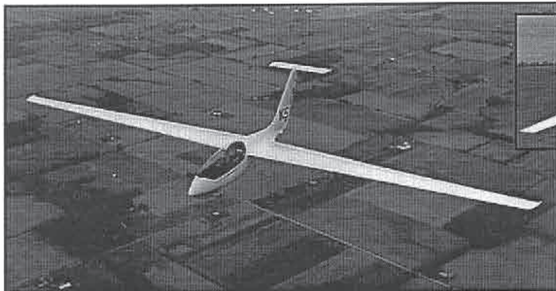
This photo shows the high aspect ratio "thresher" vertical stabilizer and sleek fuselage shape.
