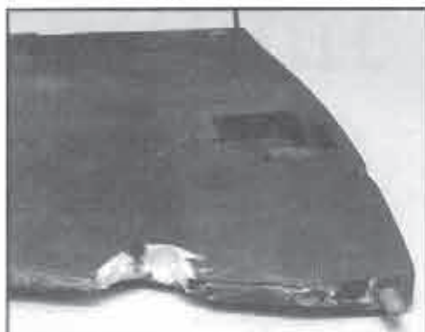
BAe Hawk wing showing Point of the Mountain "ironweed" damage and general wear.
