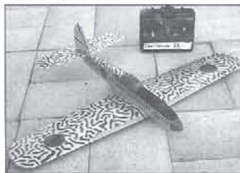
DAW Hien mini foamie equipped with Hitec 555 micro receiver and a pair of HS-85 mini tough-guy servos. Span, 30-inches, weight 9.2 ounces, finished in Goldberg Ultracote.
