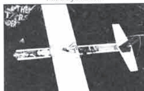
Close up of the Blue Foamie's innards. Brad's version uses a bit more wood than an out of the box. Note the ply motor bulkhead/motor mount and 1/64" ply used on the wing to handle the rubber band "rash". Can't get much simpler!!
