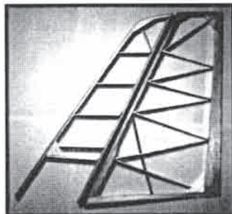
The finished fin and rudder, with modified tip outline. This modification did not change the overall area. The flexible hinge is glued in place after covering.
