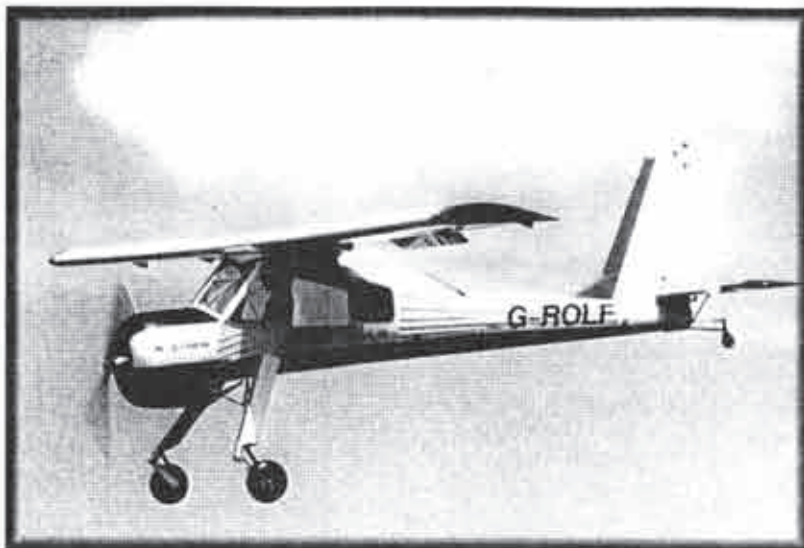
The gentle giant 1/3 Wilga stands waist high. Perhaps the easiest of towplanes to fly and land, it's powered by a King 140 twin up front, and will tow the very largest of sailplanes with ease.
