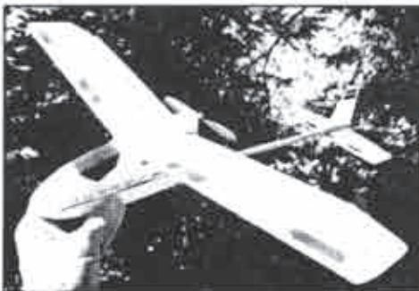
The free flight, Skybot, can be put together in just a few minutes. Its little motor can be charged with an external battery pack. It's best flown in a large, open area, because it flies a long way. Excellent for beginners.
