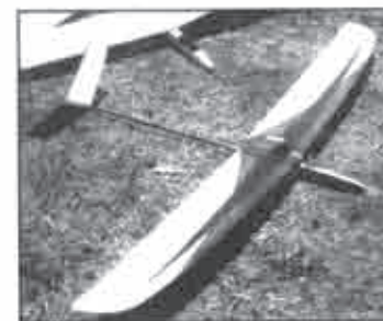
(R) Thermal-Gromit Works Meteor flown by Adam Weston (19th in open class), 6 oz. flying weight, SD-7003, Kevlar pod, CF boom, glass bagged wings. The Meteor is launched by a wing tip side arm throw which results in a very competitive launch. The Meteor may be released as a kit. [www.tgworks.com]
