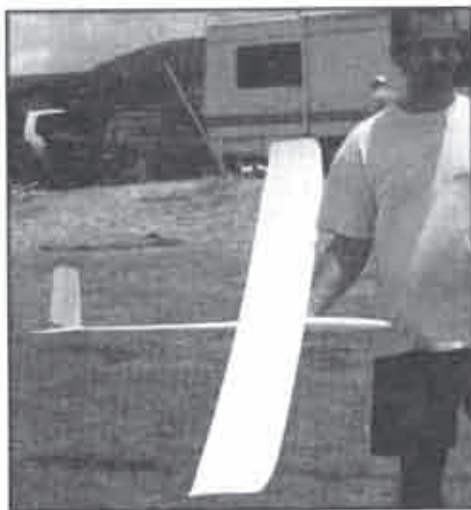
Ralph Mittelbach with his hollow molded design. Two channel poly with constant chord wing, tripped SD-7037, molded finger hole, balsa tail surfaces and curved up tips as often seen on current F3J designs.
