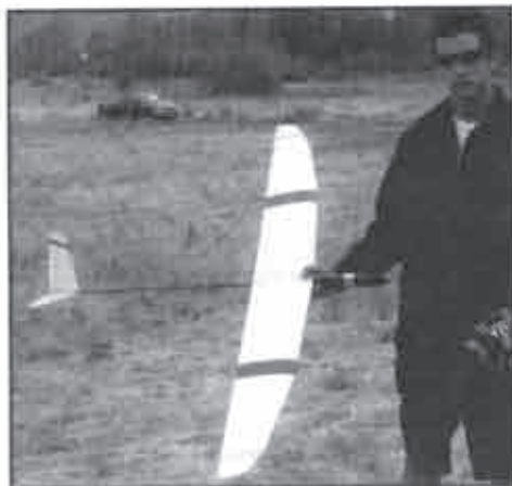
Paul Anderson with Leza. Stock NSP Psycho wing with own design fuselage and tail. Weight is 9 oz. with four servos. Regarded by many at the '99 IHLGF as the highest launching man-machine combination.
