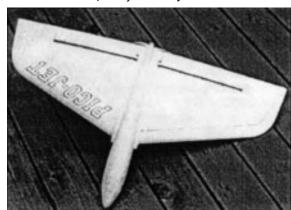
Underside of Pico Jet - bright band forward of elevons is reflective tape added for ID purposes.
