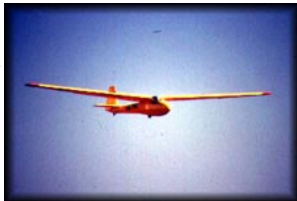
(Above & Below) David Crutchley of Bloomington, IL brought a Flair 1/4 scale ASK-8b for his first aerotow event. Model is all built up with 144" wingspan and 7.5 lb. flying weight.
