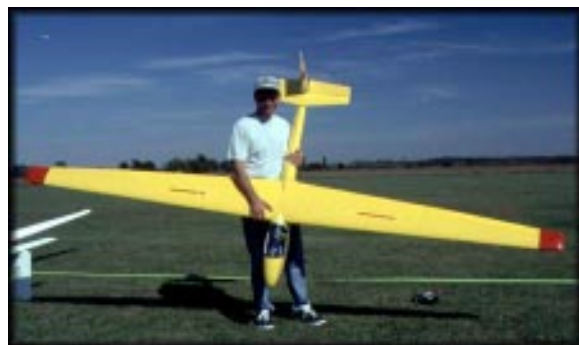
(Above & Below) David Crutchley of Bloomington, IL brought a Flair 1/4 scale ASK-8b for his first aerotow event. Model is all built up with 144" wingspan and 7.5 lb. flying weight.
