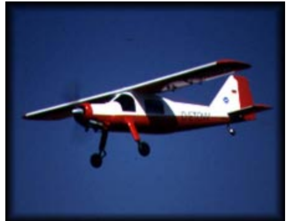
Event director Peter George's workhorse tug - a 1/4 scale Vogt Modelbau Dornier Do27. Powered by a 70cc Brison motor and weighing in at 32 lb., this model easily handled 185 of the 201 tows made during the event.
