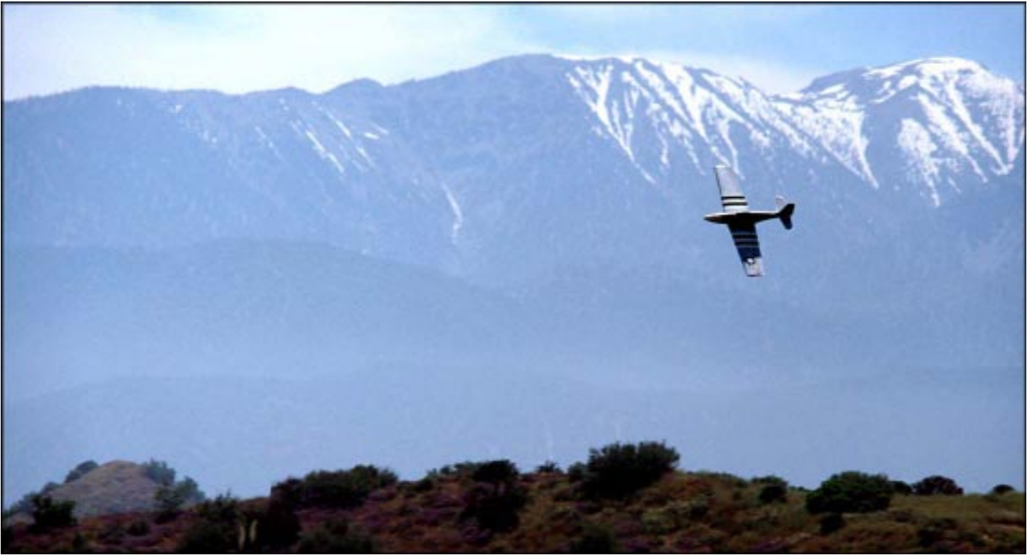
Patton Aircraft EPP-foam P-51 Mustang. Steve Patton is known for thinning the wings for reduced drag and increased speed. His slope planes are kitted by Patton Aircraft.
