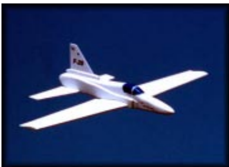
Steve Greenfield's new "Monster Tigershark." A 60-inch span slope jet carved from EPP-foam, this plane flies very well and will be made available as a kit by California Sailplanes.
