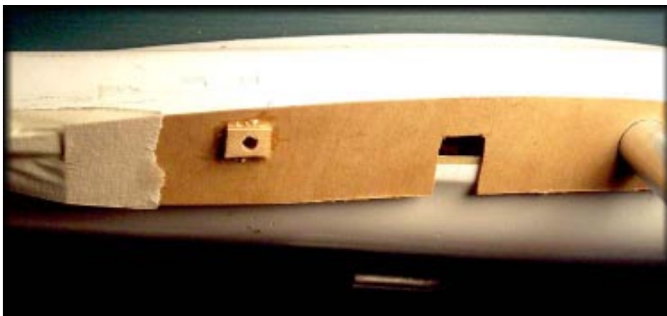
Plywood template in place ready for drilling.
