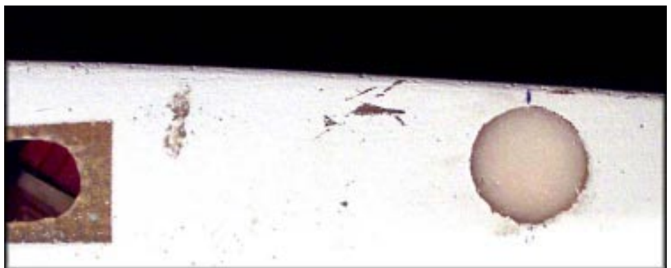
Re-filled hole ready for drilling.
