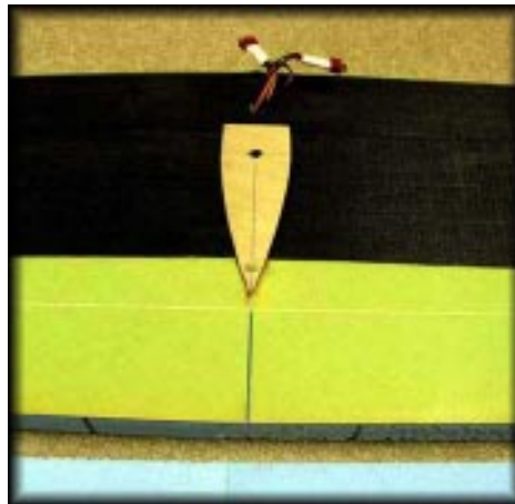
The bottom of the center section. The piece of plywood sits on top of the pylon with a metal bolt holding the wing on, and a plastic alignment bolt at the back. If the wing tip impacts something the wing will rotate on the hold-down bolt and break the alignment bolt, hopefully saving the wing, and the pylon. This design feature does a lot to reduce damage on hard landings, mid-air and inadvertent tree landings.
