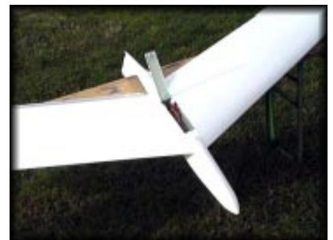
Access hatch open. The spar system does not produce any obstruction and all servos are mounted in the wings.
