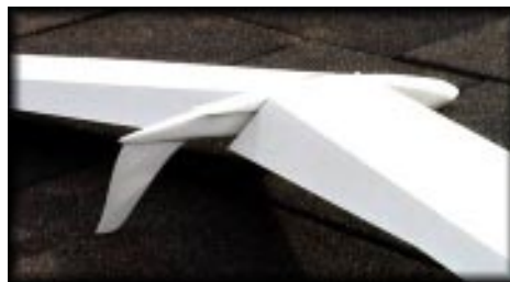
The huge flaps are fully deflected in this photo. The sub fin drives the wing to a negative angle as soon as the aircraft touches the ground, eliminating any bouncing.
