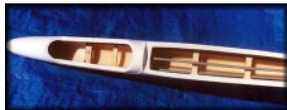
Servo mounts, pushrod tube and antenna tube, all factory installed.
