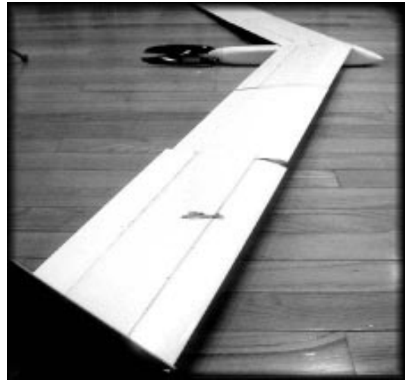
Close-up of the LE flap system on KU2F5Fv.1.
