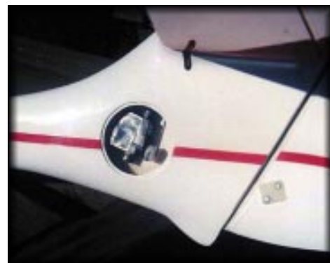
JR 241 elevator servo. A bit tricky to install.
